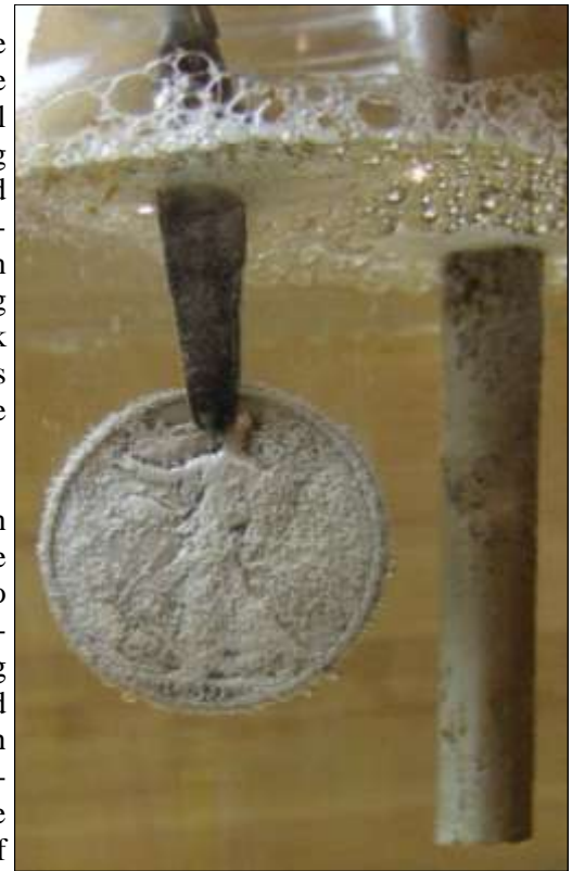
Hydrogen bubbles being released
